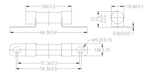
Note: recommend tightening torque is 3.5-4.0Nm.
